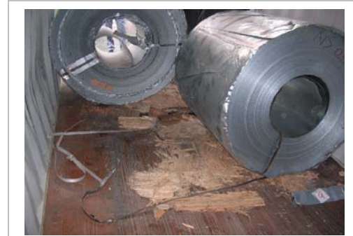
Loose coils, breaking floor and panels
