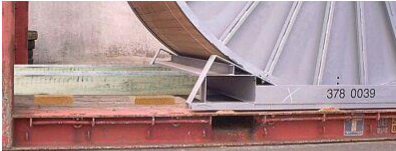
Lengthwise securing using squared lumber
