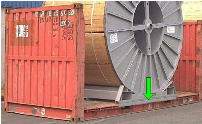
Lateral securing using steel edge provided at the design stage
