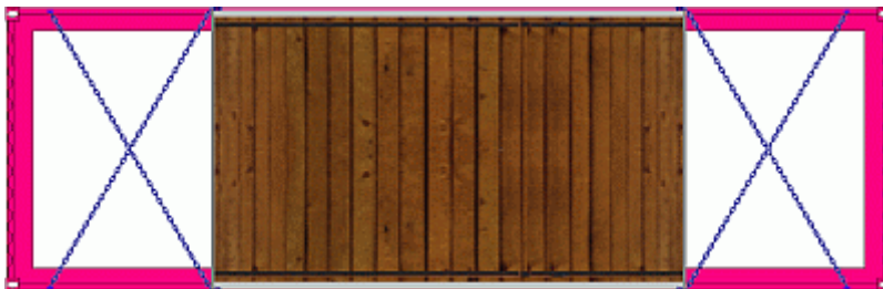
Lengthwise and transverse securing using chains - plan view
