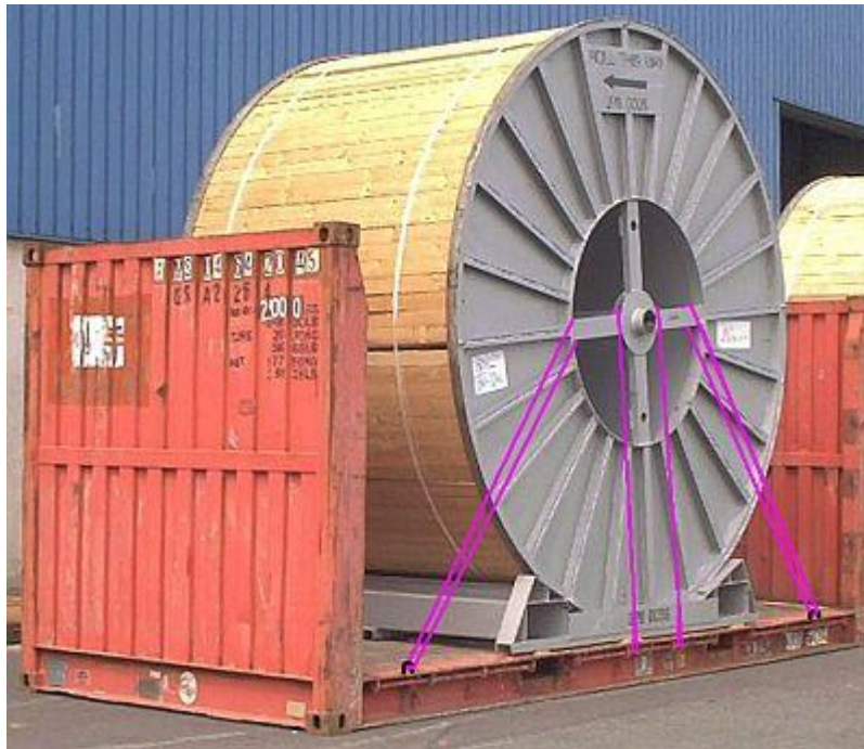
Vertical securing and securing against tipping using vertical and oblique lashings
