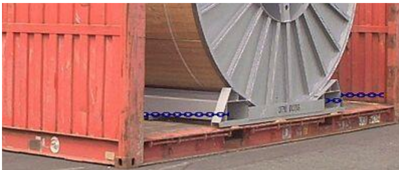
Lengthwise and transverse securing using chains
